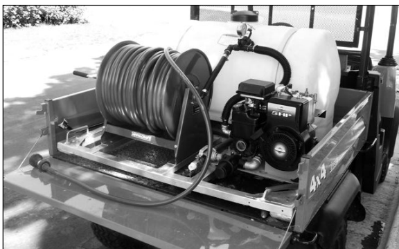
New Water Pump on Preserve Utility Vehicle (D Einstein)
