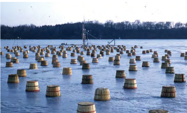
▲ The change in wind speed was measured by placing bushel baskets on ice—first far apart, then close together, then piled on top of one another.
